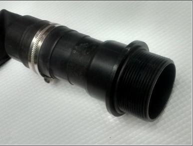
Insert the other side of the sleeved inner-tube into the other tank connector.
