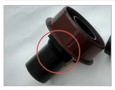
Insert the 10 cm pipe on both sides of the tank connector that are still not used (external side)
