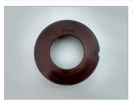
Drill the centre of the two 110 mm socket plugs using the 64mm hole saw.
