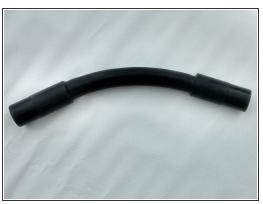
Sleeve both sides of 50cm piece of inner-tube( component 2) around the two 13 cm pipe pieces by approximately 8 cm.
