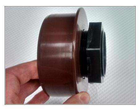
Take the 110 mm socket plug with the hole for air connector and insert one of the tank connectors.
