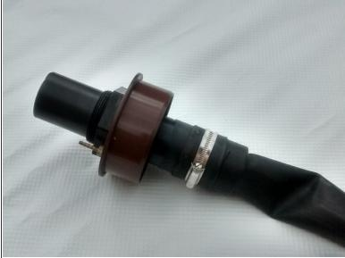
Take the socket plug with the tank connector and the installed air fitting and insert one of the sides of sleeved inner-tube into the tank connector as shown in the picture.
