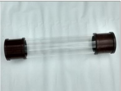
Fit the two 110 mm double socket connectors into the 110mm acrylic pipe.
