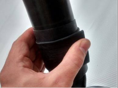
Wrap one 35cm flat piece of inner tube (Component 1a) tightly on top of one side of the previously sleeved inner-tube (from Step 11).
