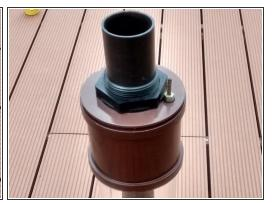
With the acrylic pipe standing horizontally insert the socket plug with the air connector (attached to the sleeved component) into the acrylic pipe
